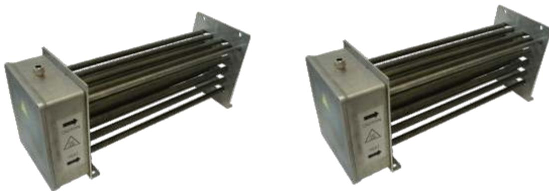
GRT style resistors are medium to high power resistors for constant load as in Filter applications and long braking cycles (example cranes). The GRT is constructed with Ø16mm tubular resistor elements, banded in U-shape and welded into two supports. On one side there is the electrical connection box in IP65 or higher.
