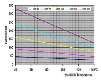
This graph shows the maximum wattage rating for each of the five possible ressistors of standard size corresponding to the heat sin temperature. It is assumed that all resistors are equally loaded.
