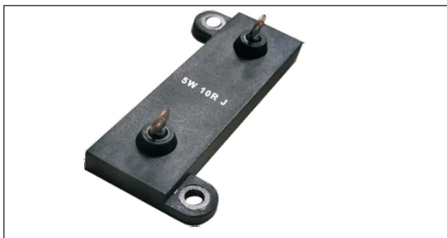
Manufactured in cermet thick film technology, these power resistors exhibit remarkable characteristics and the series includes 4 types ranging from 5 W to 50 W. Designed to be mounted onto a heatsink, the resistor can bear high short time overloads and 3 types of terminations are available. The resistors are non inductive and are particularly suitable for high frequency operation and cut-out circuits.
